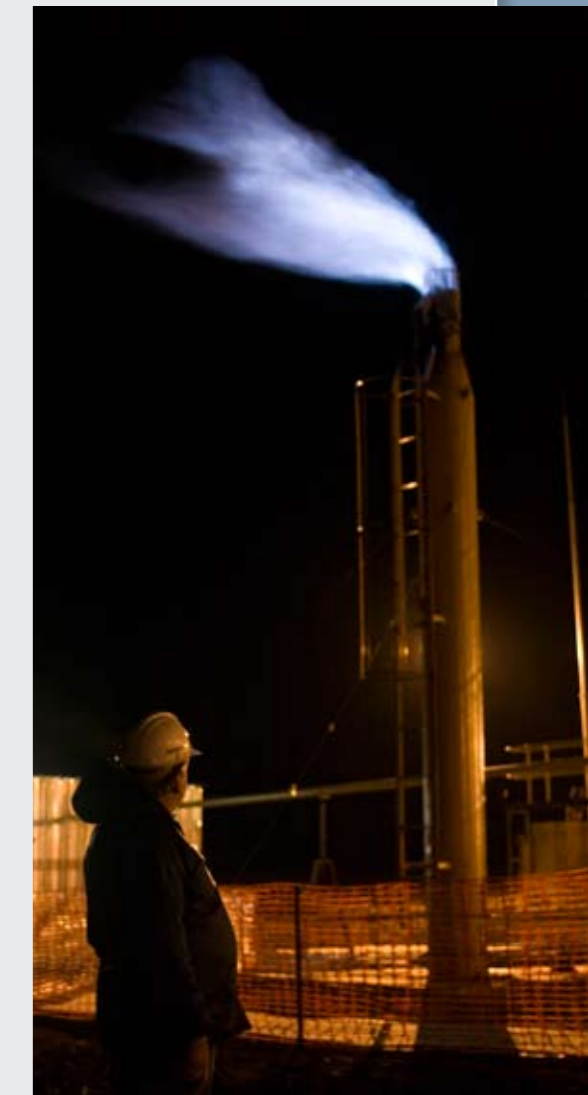
A successful flare at the underground coal gasification pilot plant at the Majuba power station.
